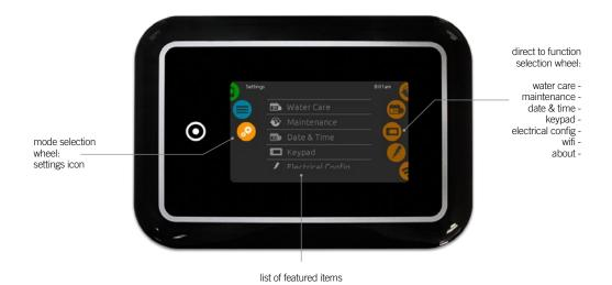
To select the settings mode, slide the left wheel up or down until the settings icon menu is highlighted in the middle.
