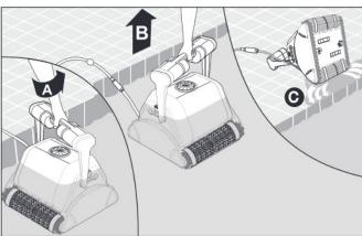
Using the Bating cable, bring the Pool Cleaner to the pool's edge.
