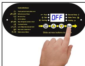
Heating / Cooling modes only available on select equipment. Confirm chiller features before setting a mode.
