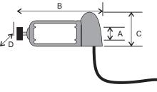
Approx. trigger range: Contact will trigger (close) when magnetic float present (within range A).
