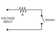
High surge currents may cause damage to the sensor and significantly reduce its life, the following circuit is, therefore, highly recommended.
