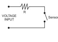
High surge currents may cause damage to the sensor and significantly reduce its life, the following circuit is, therefore, highly recommended.
