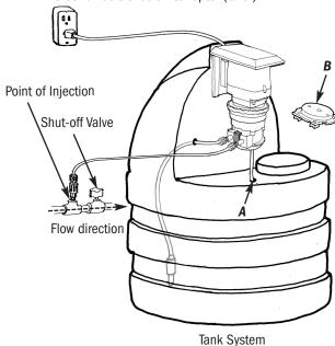
IMPORTANT! The Tank System is equipped with four screws installed into each side of the mounting bracket to prevent damage during shipping. Please remove the screws upon installation so that the pump may be easily removed from the mounting bracket when required.
