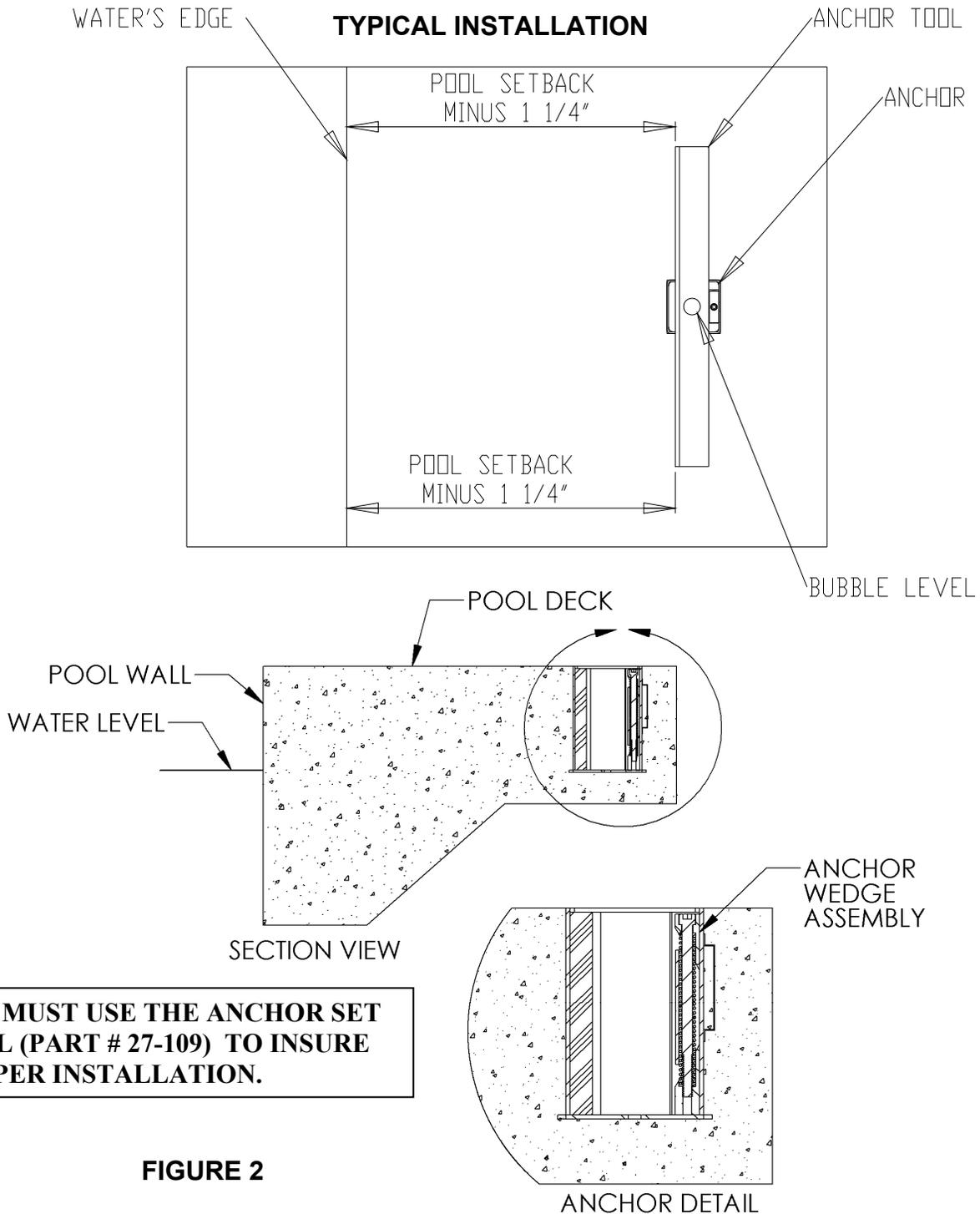
**YOU MUST USE THE ANCHOR SET TOOL (PART # 27-109) TO INSURE PROPER INSTALLATION.**
