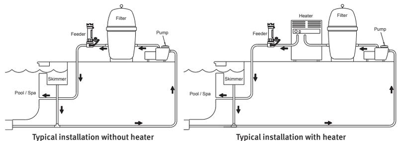
**WARNING** Do not install chlorinator into copper plumbing. Pipe damage could occur. Never install chlorinator before heater. Heater damage could occur.
