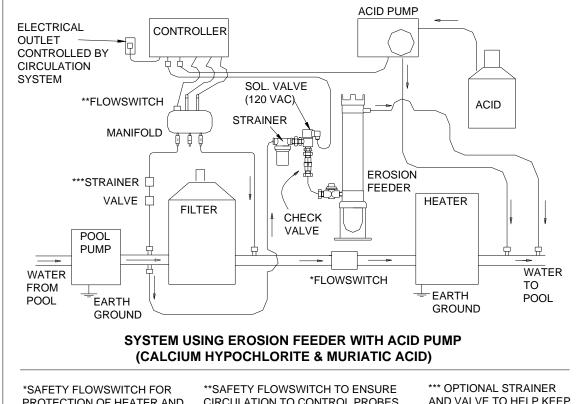
\*SAFETY FLOWSWITCH FOR PROTECTION OF HEATER AND TO ENSURE DILUTION OF CHEMICAL INTO POOL. \*\*SAFETY FLOWSWITCH TO ENSURE CIRCULATION TO CONTROL PROBES AND INDICATOR THAT POOL CIRCULATION IS OCCURRING. \*\*\* OPTIONAL STRAINER AND VALVE TO HELP KEEP MANIFOLD AND PROBES CLEAR OF DEBRIS.
