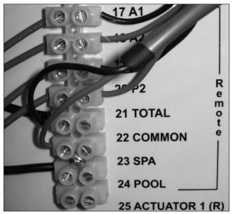
Fig. 11: Heater Wiring Block
