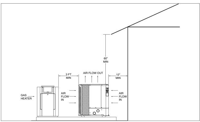
Fig. 1: Installation Clearances
