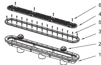
1. 32" Three-Port Manufactured Vinyl Sump Bucket With Gasket
