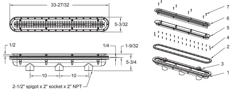
1. 32" three-port manufactured fiberglass sump bucket
