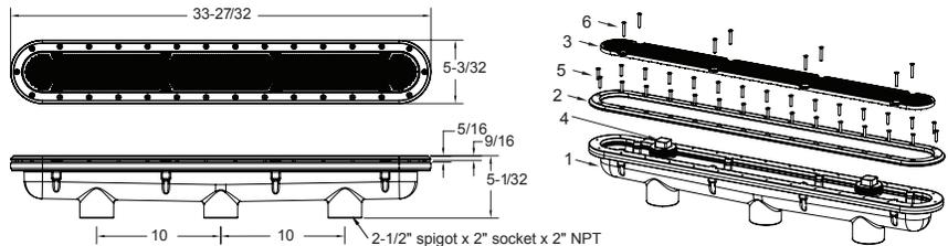
1. 32" three-port manufactured fiberglass sump bucket
