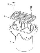
2" x 4" gutter/deck drain body
