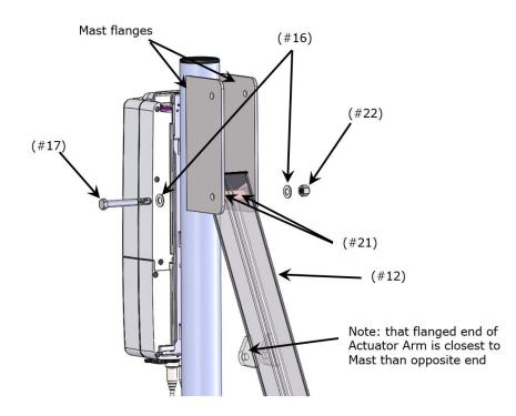
11. Verify that Actuator (#1) is already attached to base of Mast, with (1) Hex Head Bolt (#23), (2) Washers (#16), and (1) Nyloc Nut (#22).
