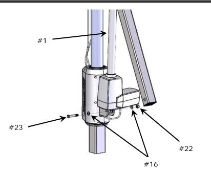
12. Attach the opposite end of the Actuator (#1) to the Actuator Arm Assembly (#12) using (1) Bolt (#23), (2) Washers (#16) and (1) Nut (#22) through the holes in the flanges of the Actuator Arm (see image below).
