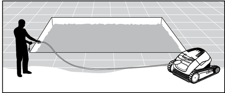
**5.1.2** Unwind the cable and stretch it out completely so that it has no kinks.
