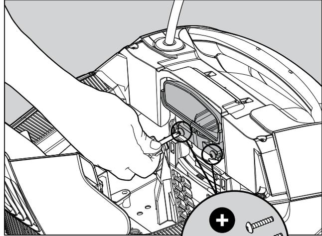
**8.1.2** Using a short screwdriver open the 2 screws.
