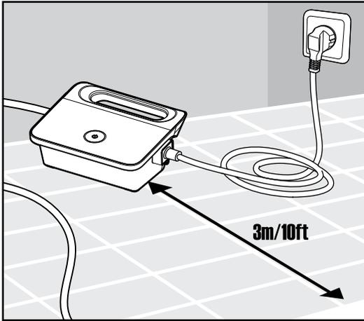
**5.1.1** Position the power supply so that it is approximately in the middle of the long side of the pool at a distance of 3m/10ft.
