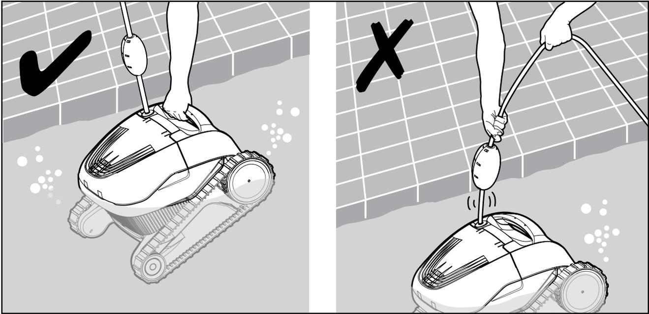
5.3.2 Using the floating cable, bring the Pool Cleaner to the pool's edge.
