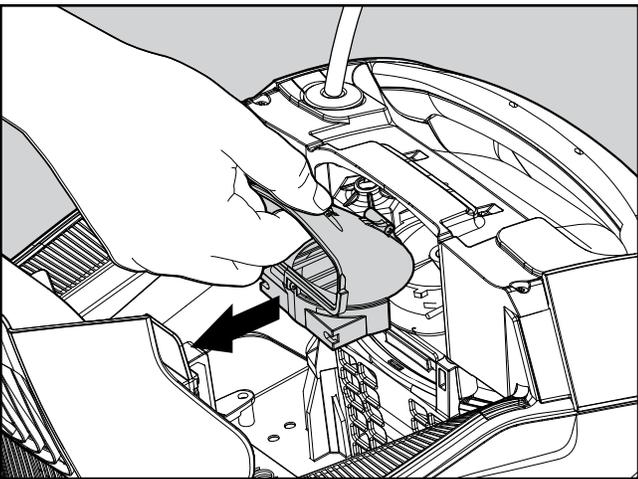
**8.1.3** Pull the impeller cover backwards to release it. Clean the debris trapped around the impeller. Assemble the impeller cover.
