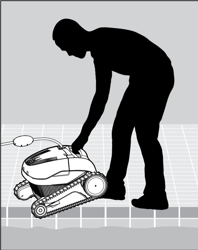
**5.2.1** Put the Pool Cleaner into the pool. Release the Pool Cleaner and let it sink to the floor of the pool. Make sure that the floating cable is free of any obstructions.
