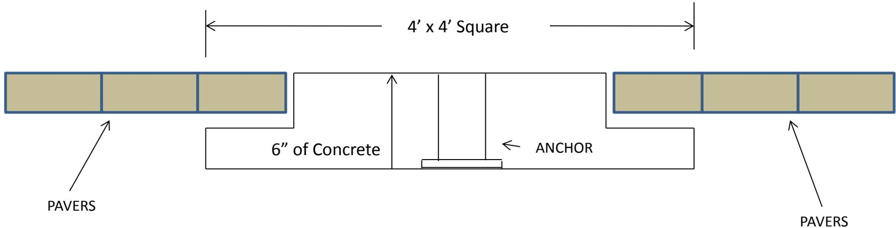
**Option #2** same as Option 1, just recess the concrete down and reinstall the pavers over the concrete except directly under the pool lift, That section needs to remain concrete!
