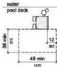
4. Submerged Depth. The lift shall be designed so that the seat will submerge to a water depth of 18 inches (455 mm) minimum below the stationary water level. To make sure the lift has enough clearance the lift should be installed at a location with 48" of Water depth
