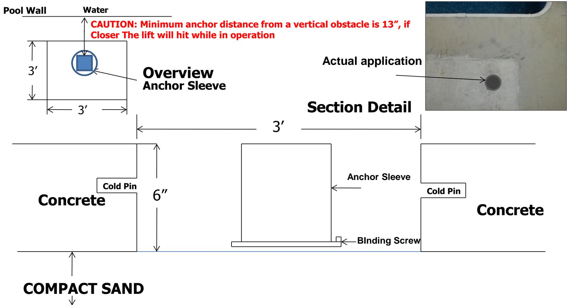
Front of Anchor Sleeve must be 12" to 36" from the water's edge or 13" min if an obstacle is present before the water. Connect the binding screw to your bonding grid
