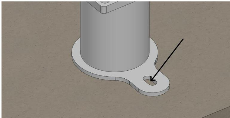
Now mark the concrete so you will know where to drill (the hole should be centered in the slot).
