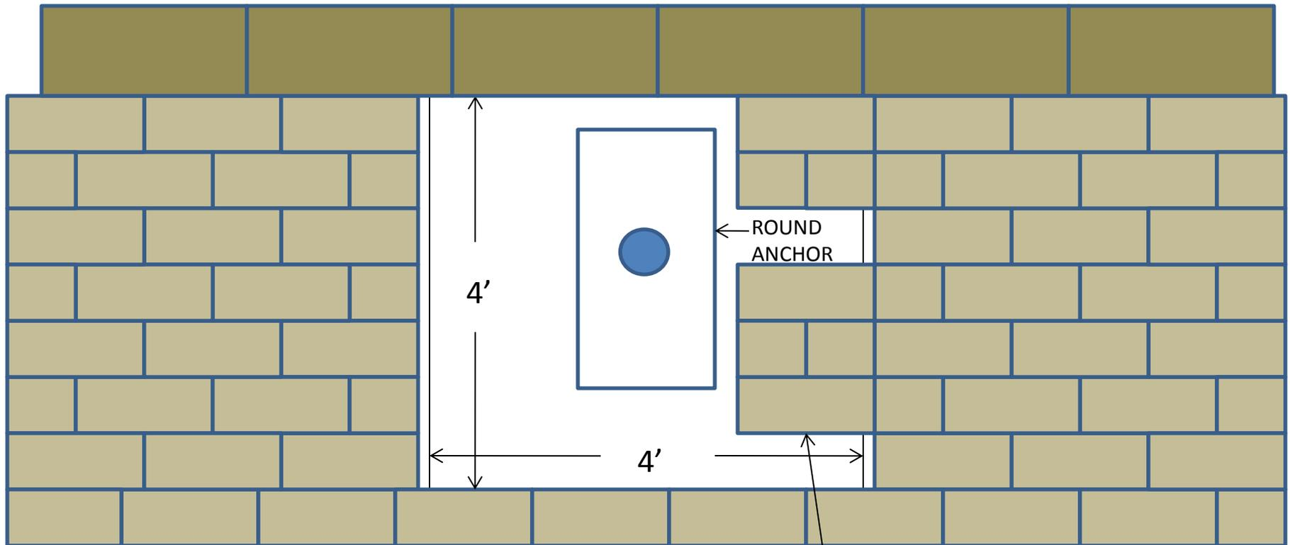
**Option #2** same as Option 1, just recess the concrete down and reinstall the pavers over the concrete except directly under the lift, That section needs to be concrete
