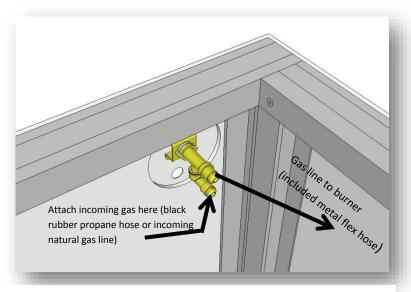
Do not make gas connections to burner until concrete top is installed. Gas connections can be made from below or from above by lifting burner to access gas line.
