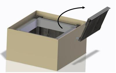
2. Set the base in the desired location and set top onto base. Ensure top is aligned with the wood dowels, found in each corner. Replace access door.
