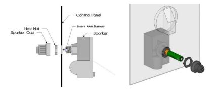
6. Connect sparker wire and ground wire from burner to sparker box as shown below. Ensure good contact between connections. Test sparking system by pressing the button and listening/watching for the spark between the electrode and sparking tab at the burner surface. Consult the troubleshooting section of the Crystal Fire Manual if spark is weak, intermittent, or not present.
