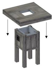
Using a power drill and Self Tapping Philips Head Screws provided, attach Top Attachment Brackets to secure WP-TILETOP to WP-BASE as shown in the figure below. Secure each attachment bracket using 4 screws.
