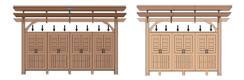
7. Fasten the TOP RAILS with 1.5" SCREWS as shown.
