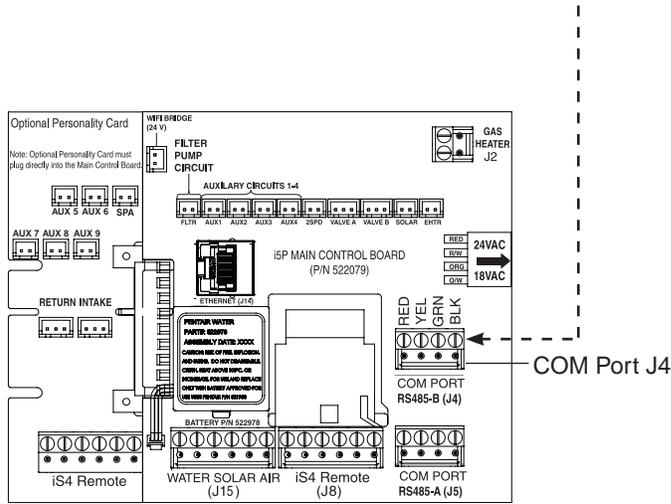
IntelliCenter Control System main circuit board (with i10PS optional expansion card shown)
