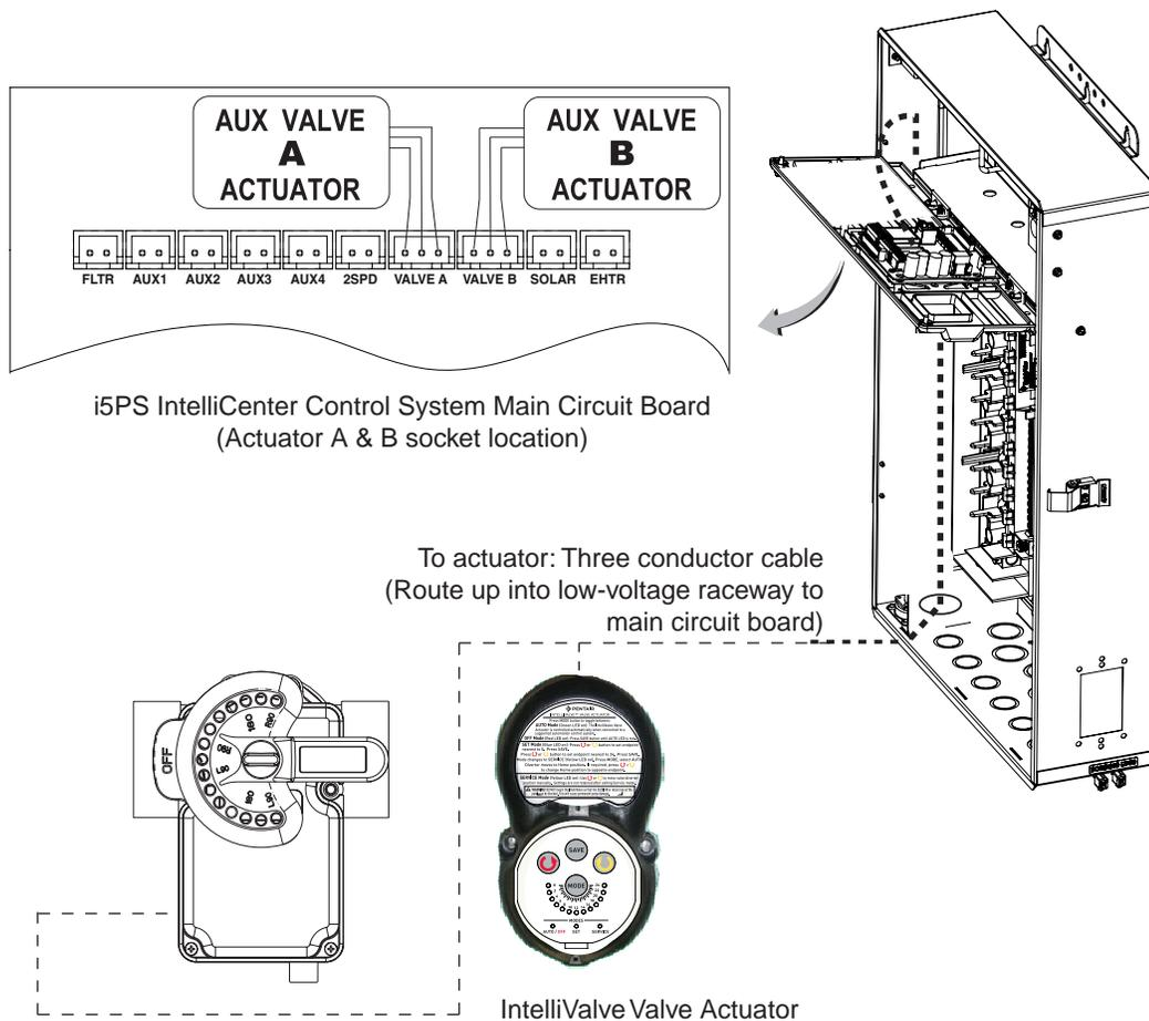
Note: Connect the IntelliValve Valve actuator to AUX Valve A or Valve B on the IntelliCenter Control System Personality circuit board.
