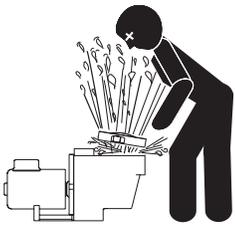
**HAZARDOUS PRESSURE: STAND CLEAR OF PUMP AND FILTER DURING START-UP**
