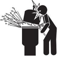
Install all electrical controls at equipment pad, such as on/off switches, timers, and control systems, etc. to allow the operation (start-up, shut-down, or servicing) of any pump or filter so the user does not place any portion of his/her body over or near the pump strainer lid, filter lid or valve closures. This installation should allow the user enough space to stand clear of the filter and pump during system start-up, shut down or servicing of the system filter.
