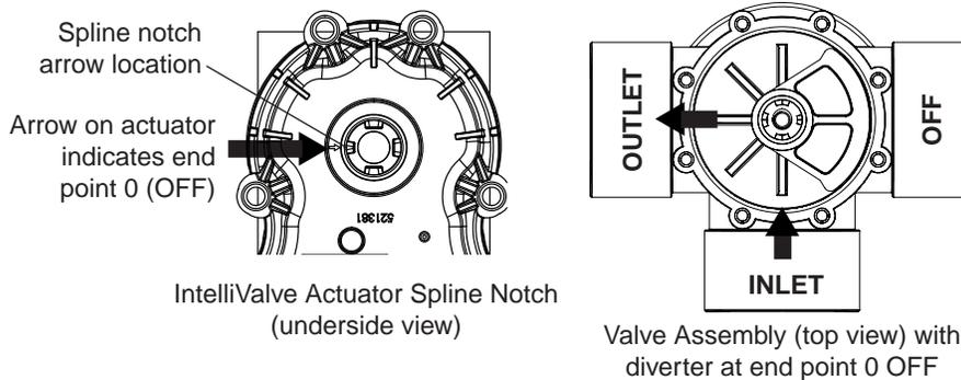
3. Mount the IntelliValve valve actuator onto the valve assembly and secure it with the four 2¼ inch mounting screws provided, as shown on the next page.
