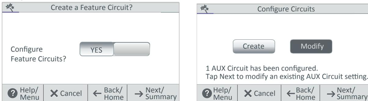
**Create / Modify:** Tap Next after the first AUX Circuit has been configured. The Configure Circuits screen is displayed. Select either Create or Modify to create a new circuit or modify an existing AUX Circuit. After you have configured all of the available AUX Circuits, tap Next to continue to Configure Valves.
