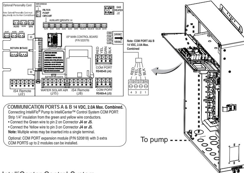
**COMMUNICATION PORTS A & B 14 VDC, 2.0A Max. Combined.**
