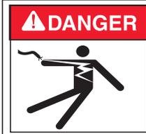
**TO AVOID AN ELECTRICAL HAZARD - Do not connect the power source conductors to the Load Center circuit breaker until all electrical connections for all loads (heaters, pumps, motorized valves, and lights etc.) have been completed.**
