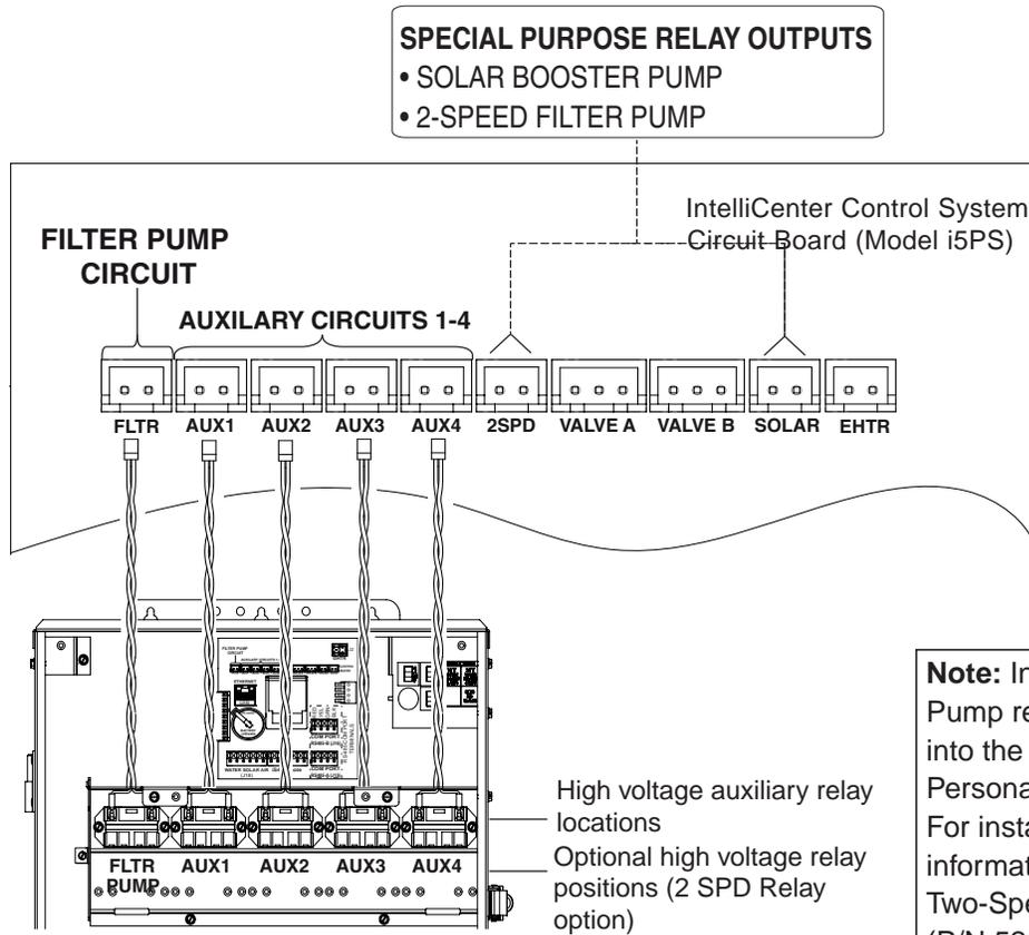
IntelliCenter Control System Load Center relays AUX circuits connections (i5PS model)
