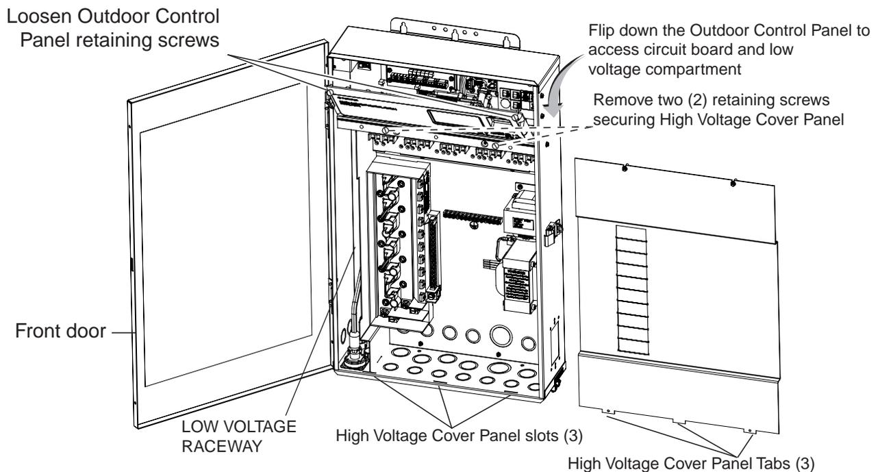
IntelliCenter™ Load Center Control System Load Center (front view)
