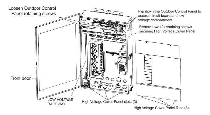
IntelliCenter<sup>™</sup> Load Center Control System Load Center (front view) (High Voltage Cover Panel removed)
