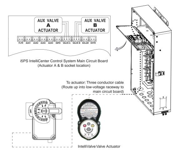
Note: Connect the IntelliValve Valve actuator to AUX Valve A or Valve B on the IntelliCenter Control System Personality circuit board.
