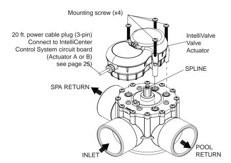
CAUTION: DO NOT mount the IntelliValve so that the suction or return line of the pump can be blocked. This will cause permanent pump damage.
