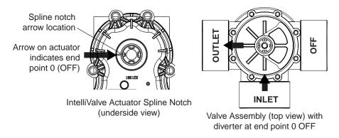
3. Mount the IntelliValve valve actuator onto the valve assembly and secure it with the four 2½ inch mounting screws provided, as shown on the next page.
