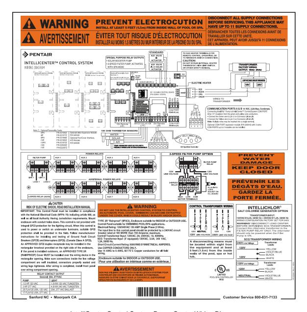
IntelliCenter Control System Power Center Wiring Diagram
