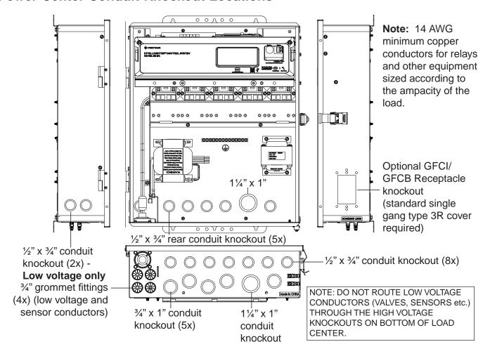
IntelliCenter™ Control System Power Center (Lower, side and back panel knockout locations)
