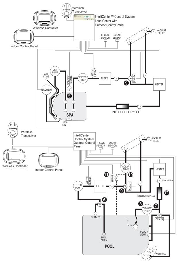
Recommended Hydraulic Schematic for Single Body Systems
