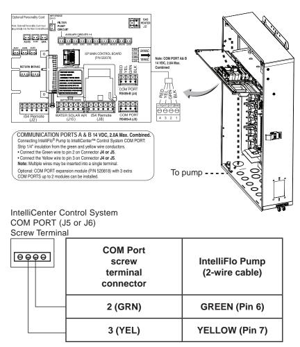
IntelliFlo pump communication cable pin out
