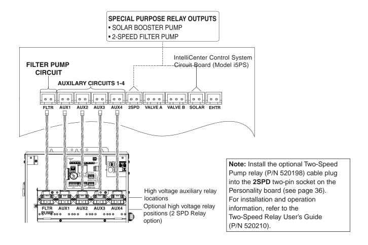
IntelliCenter Control System Load Center relays AUX circuits connections (i5PS model)
