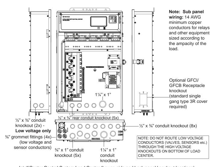
IntelliCenter Control System Load Center (Lower, side and back panel knockout locations)
