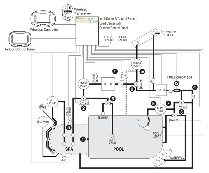
Recommended Hydraulic Schematic for Shared Equipment System
