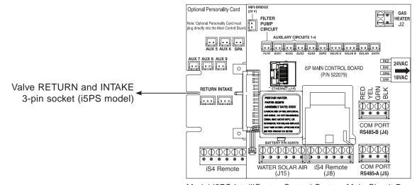
Model i5PS IntelliCenter Control System Main Circuit Board
