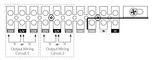
\*Note: DO NOT use or bridge both the 12VAC and 13VAC terminal positions at the same time.
