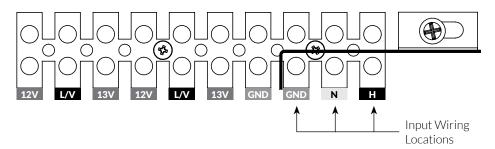
6. Replace and secure the metal input voltage isolation barrier and verify that the input wiring screw terminals are secure.
