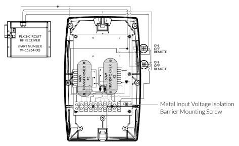
\*Note: Once all conduits are connected, replace the metal input voltage isolation barrier and mounting screw. Tighten until the mounting screw is secure.
