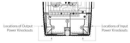
3. Using a hole saw, open the knockouts for the size of the conduit (3/4" or 1") being installed.
