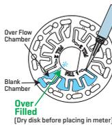
3. Do not under fill the disk. If the disk is under filled, the blank chamber will not be full. The reagent chambers will not fill entirely and results will be inaccurate.
