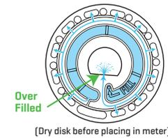
3. Do not under fill the disk. If the disk is under filled, the reagent chambers will not fill entirely and results will be inaccurate.
