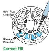
2. Do not overfill the disk. If the disk is overfilled, sample water will flow out of the vent hole in the center of the disk. The disk is not leaking. Dry the disk and run the test.
