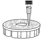
1. Fill any unused section of the disk using slow, even pressure. Add the sample water until the Blank Chamber is full and the Over Flow Chamber is partially filled.
