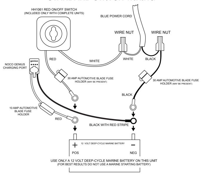
WE RECOMMEND DAILY AUTOMATIC CHARGING AT A MINIMUM 6AMP OUTPUT OR MAXIMUM 12 AMPS - FOR BEST RESULTS, DO NOT TRICKLE CHARGE
