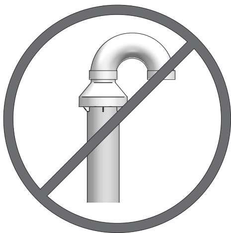
Figure 5-5 Do Not Install U-Bend to Rain Cap
