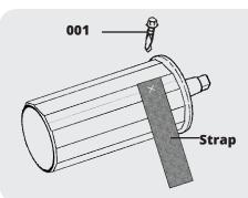
Using Tek Screws, secure the strap to the tube. Make sure you put the screw about an inch into the strap to prevent tearing.
