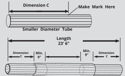
Insert smaller diameter tubes into the large diameter tube, up to the Dimension C mark, as shown. The total length of the tubes should be approximately equal to the corresponding value in Column B. See example on reverse.
