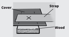
Position the blue strap on the cover. Cross cut through the strapping and the cover. Ensure that the hole in the strapping is at least 1" from the end of the strap and that the hole in the cover is at least 2" from the end of the cover. If possible fold the edge of the cover over so that you put the grommet through two layers of cover for extra reinforcement. This will ensure that the Grommet fits securely onto both the cover and the strap, and will help to prevent tearing.
