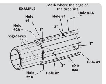
rotate 180 degrees and mark Hole #4A. This bolt will go through the same direction an Bolt #1. Drill out both holes and put the bolt through, then put the lock nut on. Now you can tighten all four bolts. Do not use an impact driver, hand tighten only. If you over tighten the bolts the tube will bend causing the bolt to stick out and puncture your solar cover.
