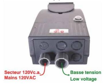
The supply box must be powered using 120V single phase current with 60Hz, and protected by a class A differential device (ground fault circuit interrupter (GFCI)), capable of providing a sufficient intensity (2A min). The cable section used for the supply must be suitable and functional over its entire length.
