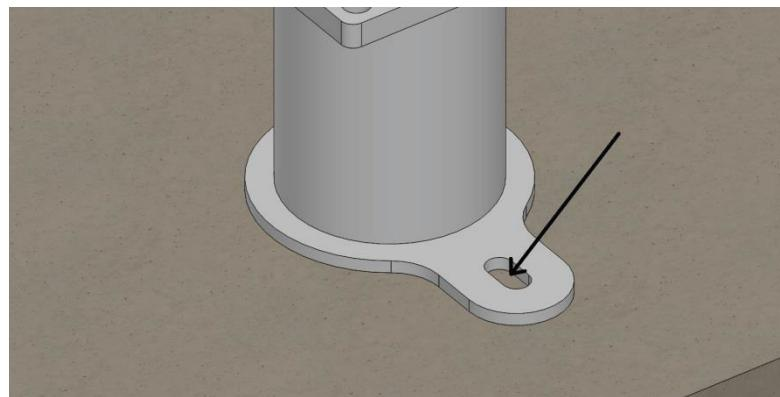
Now mark the concrete so you will know where to drill (the hole should be centered in the slot).
