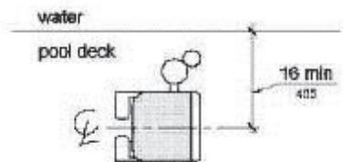
3. Clear Deck Space. On the side of the seat opposite the water, a clear deck space shall be provided parallel with the seat. The space shall be 36 inches (915 mm) wide minimum and shall extend forward 48 inches (1220 mm) minimum from a line located 12 inches (305 mm) behind the rear edge of the seat. The clear deck space shall have a slope not steeper than 1:48.
