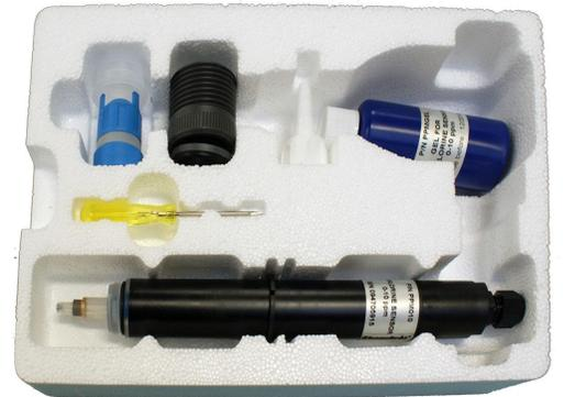
Slide the O-ring and the compression disk over the sensor tip up to the compression ring. Finally, insert the sensor with the compression fitting in the flow cell and make it finger tight.
