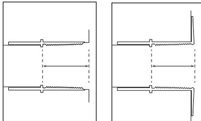
Do not install in fittings with less than 0.89" (22.6mm) of depth.
