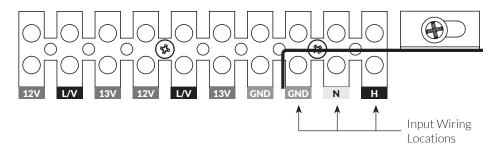
Replace and secure the metal input voltage isolation barrier and verify that the input wiring screw terminals are secure.
