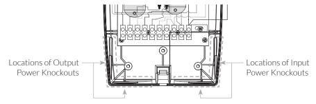
3. Using a hole saw, open the knockouts for the size of the conduit (¾" or 1") being installed.
