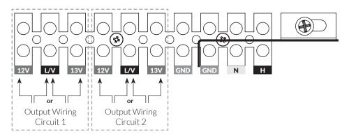
\*Note: DO NOT use or bridge both the 12VAC and 13VAC terminal positions at the same time.
