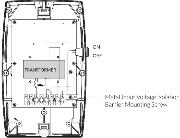
**\*Note:** Once all conduits are connected, replace the metal input voltage isolation barrier and mounting screw. Tighten until the mounting screw is secure.
