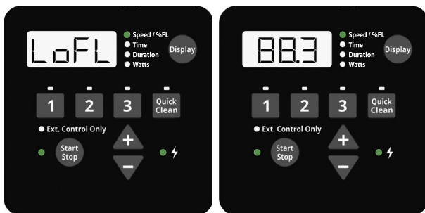
Figure 16: Low Flow Alarm
