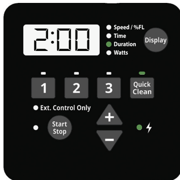
Figure 10: Setting Duration for Quick Clean
