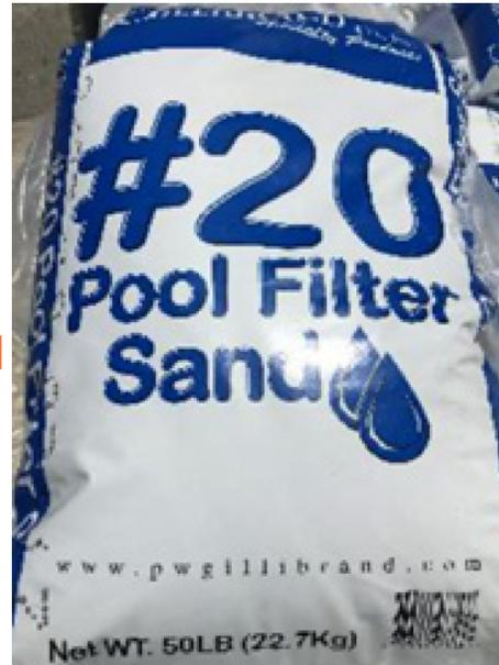
Filter sand is not beach sand. Filter sand has angular edges that capture dirt and other particulate matter. Both are limited natural resources but pool sand is mined in quarries depleting natural resources and wildlife habitat.
