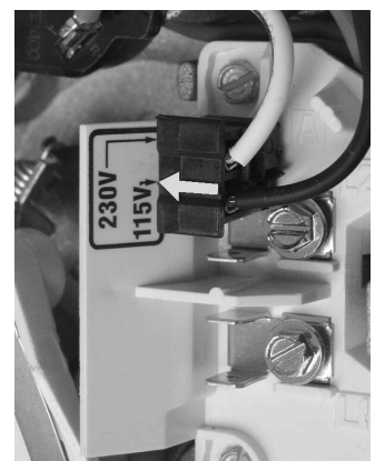
Figure 4B Voltage Change Plug Set for 115 Volts
