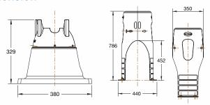
Note: MultiCyclone Support Stand is suitable for most Waterco Domestic Pool Pumps. Excluding Hydrostar & all Commercial Pumps.
