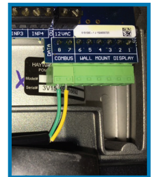
Figure 13. Pentair IntelliFlo/Hayward EcoStar Connection to Pump
