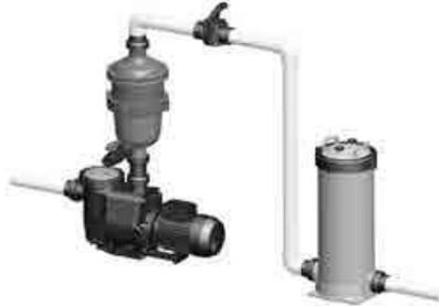
Typical Installation with a Cartridge Filter
