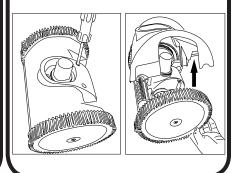
Replace the Turbine cover making sure it is on correctly Now visually inspect the rest of the cleaner removing any debris that may be in the gears, drive shafts etc. BEFORE PLACING THE SHROUD BACK ON REPEAT STEP 2 (turning the right wheel) to make sure the POOLCLEANER ™ runs smoothly. If it doesn't turn you may have replaced the vanes incorrectly. Place the Shroud back onto the POOLCLEANER ™ making sure its on correctly. Drop the three screws into the screw holes and secure.
