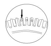
The front tires ALWAYS have HUMPS (raised treads) The back tires DO NOT have humps!
