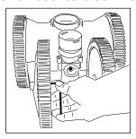
Once off, fold the tire off the Wheel Hub (step 3 above). To replace stretch the tire over the Wheel Hub (starting from one side and folding it back on). Make sure the tire is on correctly.
