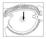
Place the bolt through the Wheel Hub line it up with the threaded hole, making sure the gear protruding from the POOLCLEANER™ engages with the gears on the Wheel Hub. Tighten bolt with Allen wrench clockwise.
