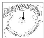
Place the bolt through the Wheel Hub and line it up with the threaded hole, making sure the gear protruding from the POOLCLEANER ™ engages with the gears on the Wheel Hub. Tighten bolt with Allen wrench clockwise.
