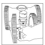
Rotate the right front tire forward to ensure that it moves smoothly. If not you fastened the wheel hub incorrectly.
