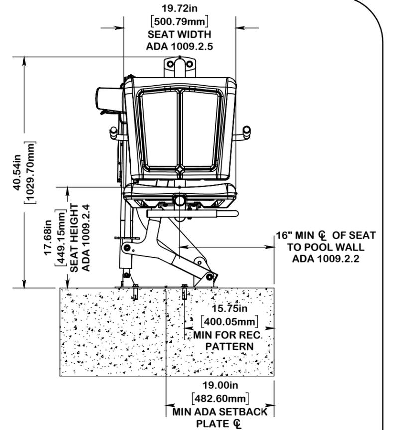
**ANCHOR PLATE DIMENSIONS; ALL HOLES FOR USE WITH 1/2" HARDWARE**
