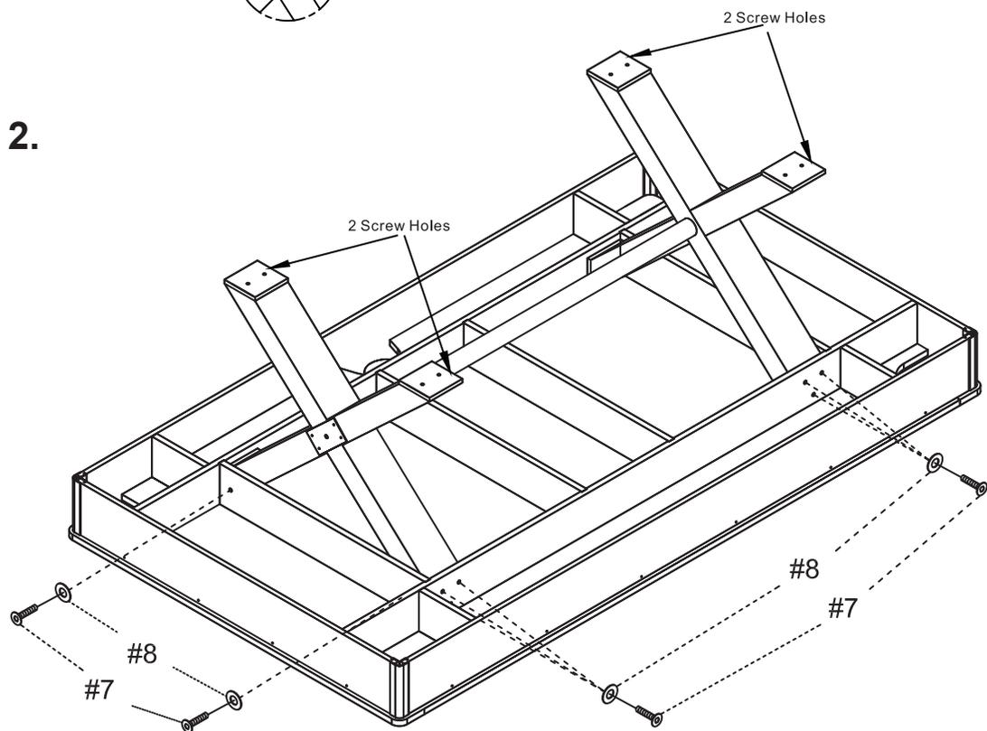
*\*Note location of screw hole positions on leg ends when assembling legs*
