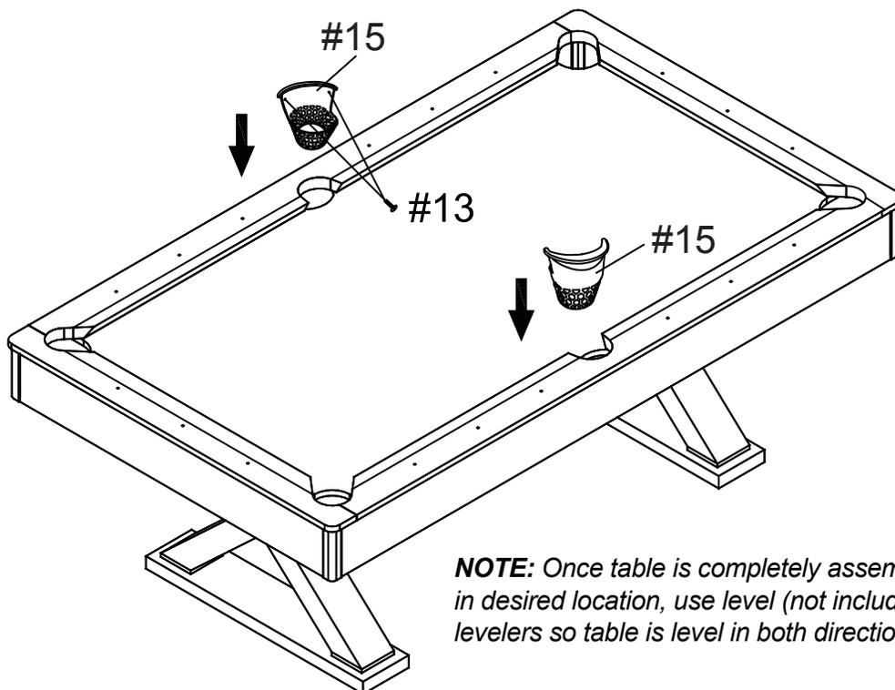
**NOTE:** Once table is completely assembled and placed in desired location, use level (not included) to adjust leg levelers so table is level in both directions.
