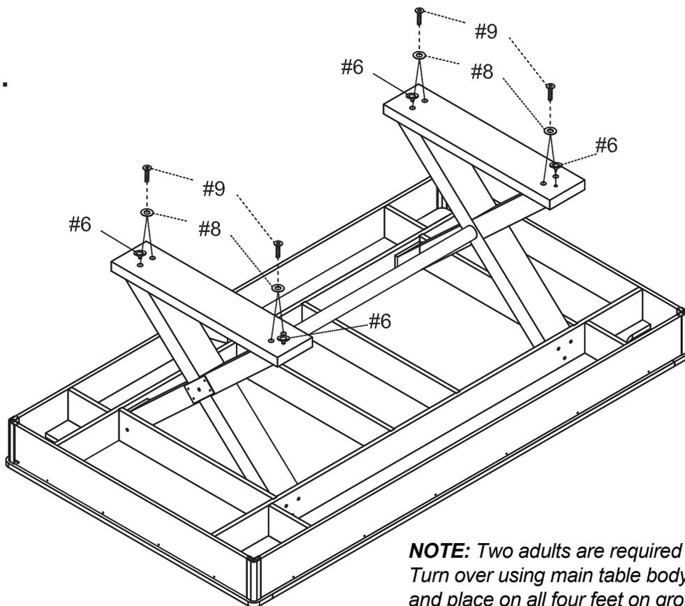
**NOTE:** Two adults are required to turn table upright. Turn over using main table body only, NOT legs, and place on all four feet on ground at same time.
