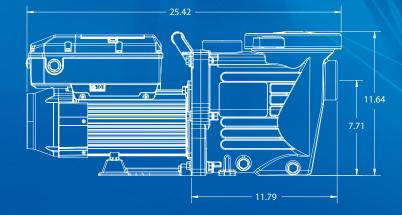
PD-140 Power Defender Variable Speed, Dual Voltage, 1.40 HP for In Ground Pools
