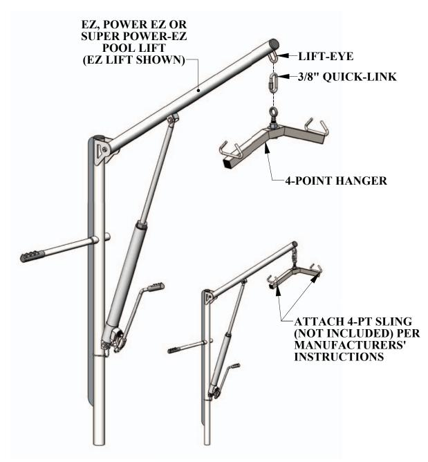
The 4-POINT HANGER BAR comes fully assembled, and only needs to be attached to the lift and sling to begin use. The 3/8" QUICK LINK goes between the lift-eye and the 4-POINT HANGER BAR eye-bolt as shown above. Be sure to tighten the nut on the 3/8" QUICK LINK to make sure it can't come off accidently.
