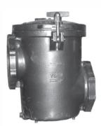
Baker Hydro introduces their new pump strainer for the series 5000 self-priming commercial pump. The strainer is designed to fit all four models of the 5000 pump series and has 6" A.N.S.I. flange connections. Strainers can also be used in line up to 50 PSI. The commercial strainer is equipped with two quick release toggle bolts for ease of maintenance and a stainless steel basket with a capacity of 440 cubic inches.
