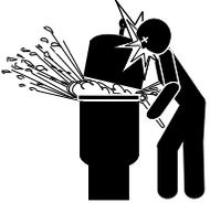
Install all electrical controls at equipment pad, such as on/off switches, timers, and control systems, etc. to allow the operation (start-up, shut-down, or servicing) of any pump or filter so the user does not place any portion of his/her body over or near the pump strainer lid, filter lid or valve closures. This installation should allow the user enough space to stand clear of the filter and pump during system start-up, shut down or servicing of the system filter.
