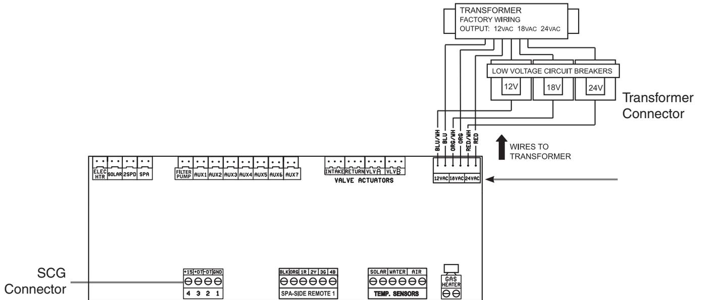
Figure 3. Transformer Connector and SCG Board Connector
