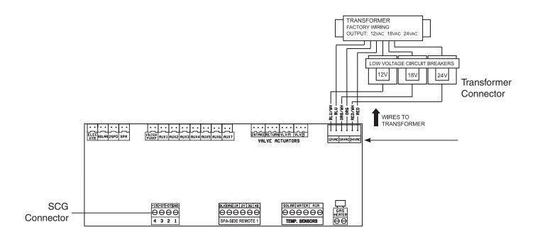
Figure 3. Transformer Connector and SCG Board Connector
