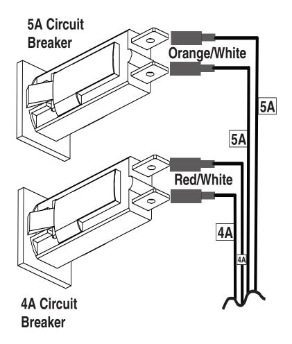
Figure 5. Circuit Breakers Transformer Connections
