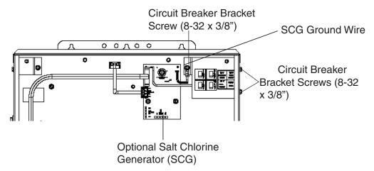
Figure 7. Circuit Breakers Bracket
