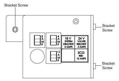
Figure 8. Circuit Breaker Bracket Screws
