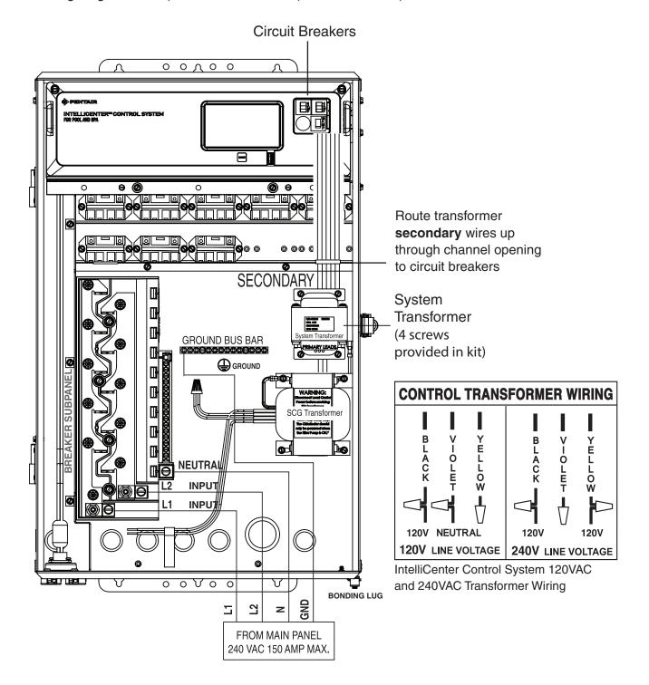
Figure 6. Wiring the System Transformer (Load Center or Power Center 2012 or later)
