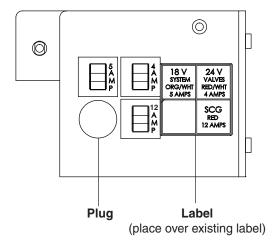
Figure 4. Circuit Breakers Wiring
