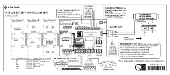
Figure 11. IntelliCenter™ Control System Circuit Board (with optional Expansion Boards shown)
