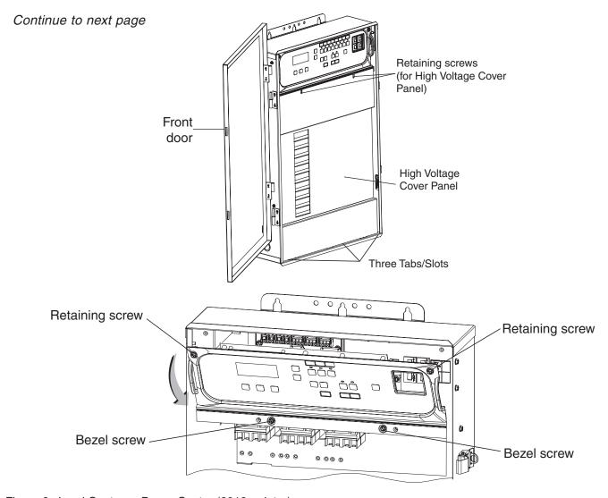
Figure 2. Load Center or Power Center (2012 or later)
