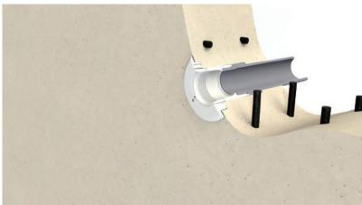
Then glue a first gasket before placing the liner;
